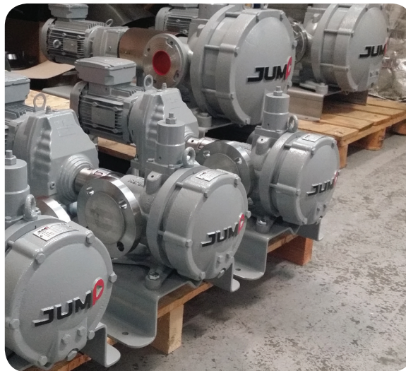
JE5c and JE36c pumping units on stationnary chassis
